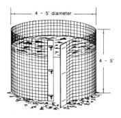
four feet high. With this design, it is easy to turn the composting material by simply unsnapping the wire or ties, moving the wire cylinder a few feet and turning the compost back into it.
